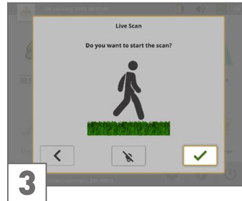
3 After the calibration has been processed the eXp 6000 ground scanner is ready to start the measurement.
