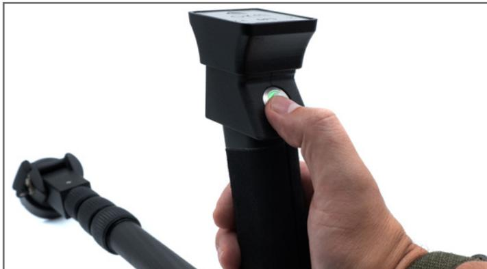
As soon as the Telescopic Rod is fully charged, remove the charger and push the Trigger Button at least 2 seconds until the LED ring of the Trigger Button lights up **green**. If the Control Unit is switched on as well, the Telescopic Rod will try to establish a wireless connection to it and – by success – the LED ring will turn **blue**.
