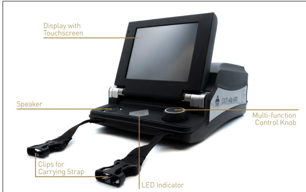
All functions are controlled by the **Multi-function Control Knob** or by using the touch capabilities of the display. To operate the device, rotate the knob to the desired function and push the knob to select it. Alternatively, simply tap with your finger onto an item on the screen.
