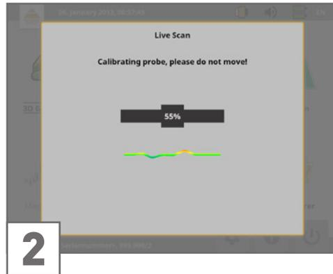
2 Now the eXp 6000 calibrates your measuring probe according to the current underground to receive optimal data afterwards.
