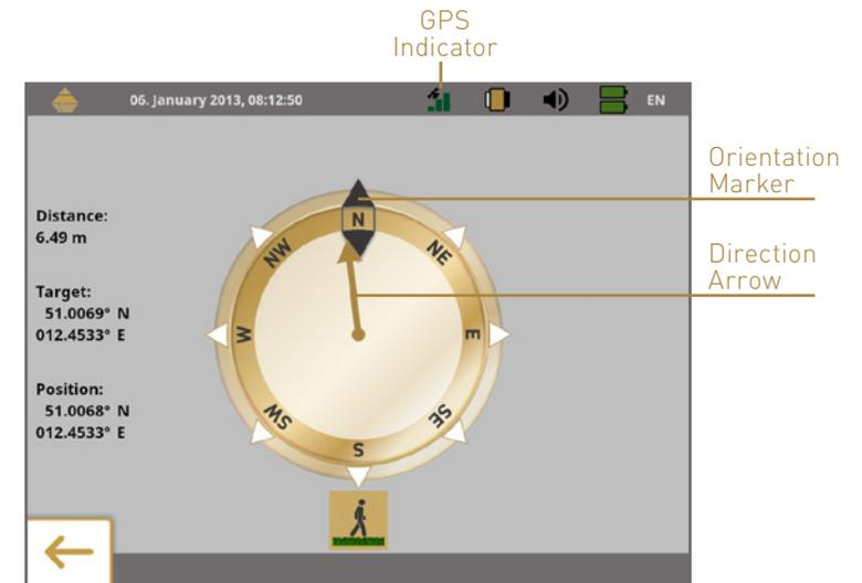
The **Position** indicates the GPS coordinates of your current position, while the **Target** is the place where you have performed your scan.
