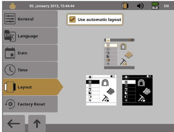
If you select the option "Use automatic layout", the eXp 6000 Control Unit selects the current layout automatically by measuring the light condition of the environment. If the light changes during operation the layout may change automatically.
