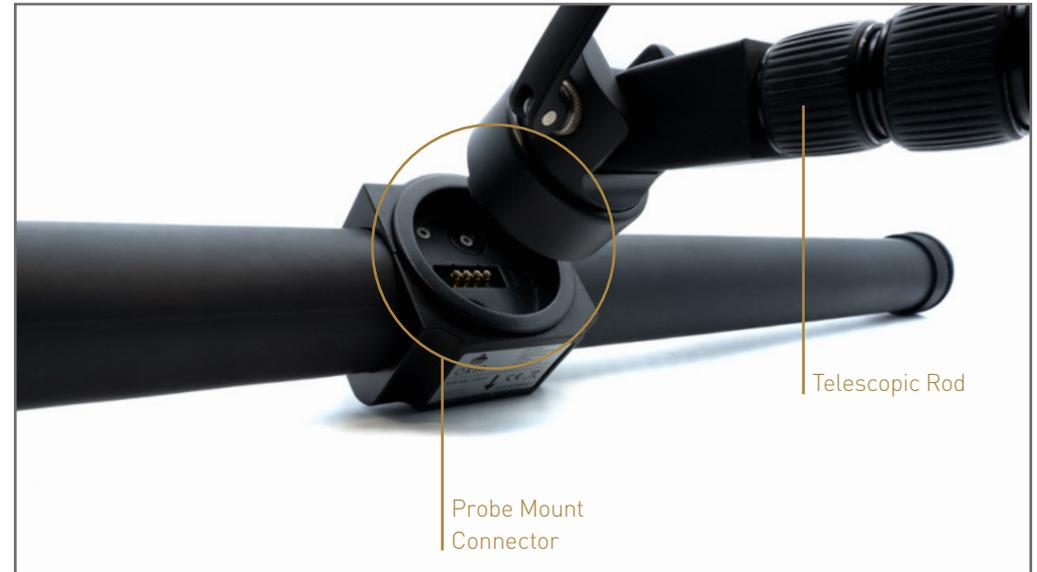
All measuring probes are equipped with a **Probe Mount Connector** that mounts the probe to the Telescopic Rod. To mount the probe, simply push it onto the probe mount of the Telescopic Rod. Thanks to the magnetic connection, the probe gets attracted in only one specific orientation to the probe mount connector.
