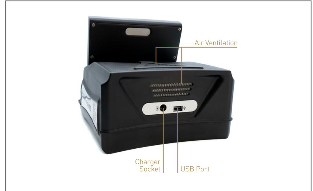
Via **USB Port** a common USB flash drive can be plugged in into the Control Unit to copy the stored scan images to another computer for further evaluation with the *Visualizer 3D Studio* software or to update the internal firmware if necessary.
