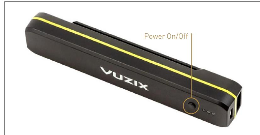
Press the Power On/Off Button on the side of the battery pod to switch on the Video Glasses. For further information please refer to the VUZIX M300XL User Guide.
