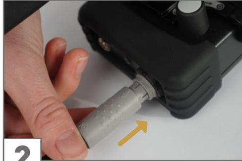
Plug the Connector of the Search Coil into the designated Socket of the Control Unit.
