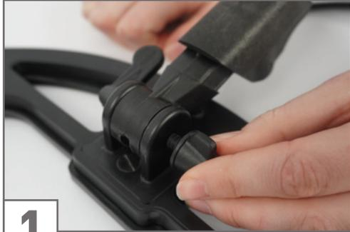
Unscrew the bolt from the Search Coil Mount of the Telescopic Rod. Make sure the rubber washers are seated next to the shaft before attaching the Search Coil.
