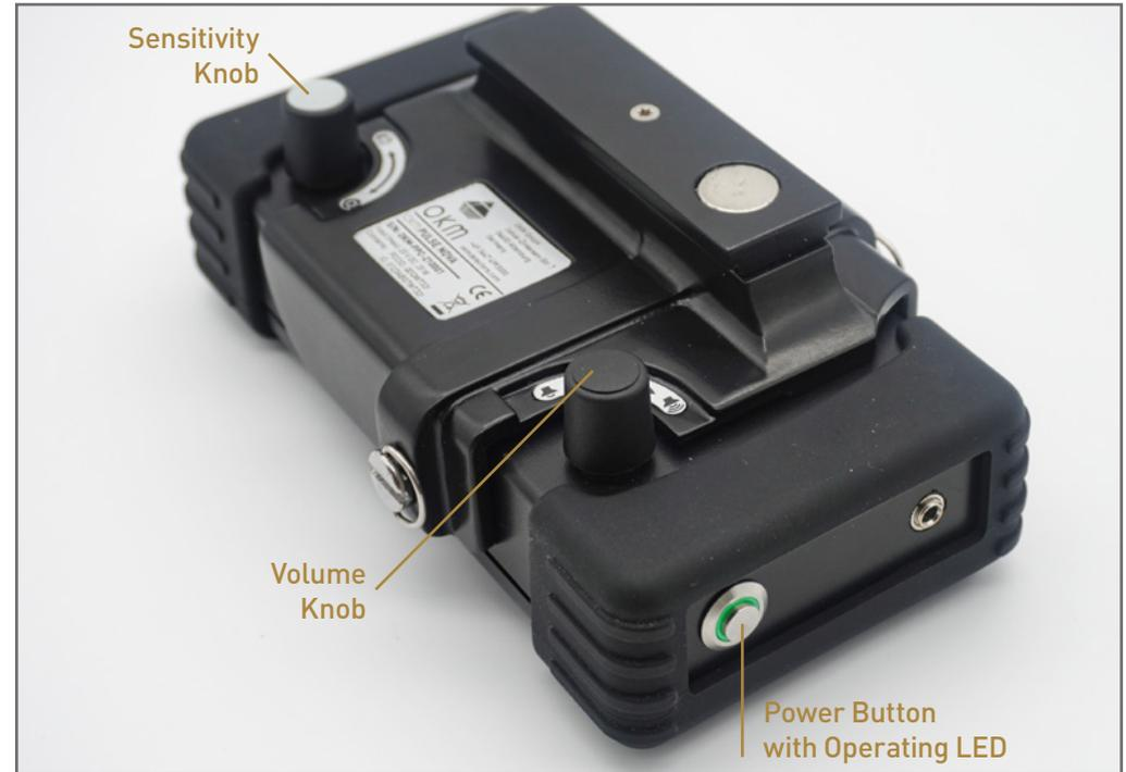
**Power Button with Operating LED:** Push the Power Button to switch on the Control Unit. At first, the Operating LED starts blinking for about 2 seconds before it remains **green** permanently. If the LED blinks rapidly before turning off, the internal battery is too low and must be charged (see chapter "4.1 Charging the Control Unit" on page 13).
