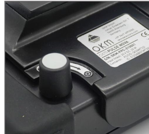
Push and hold the Sensitivity Knob of the Control Unit to start a new ground balance.
