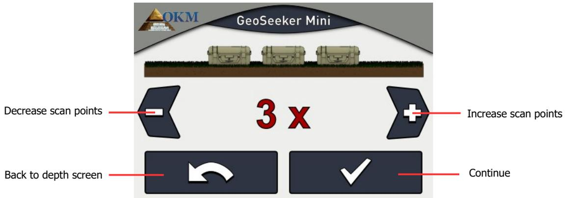
Figure 5.3: Adjusting the number of scan points
