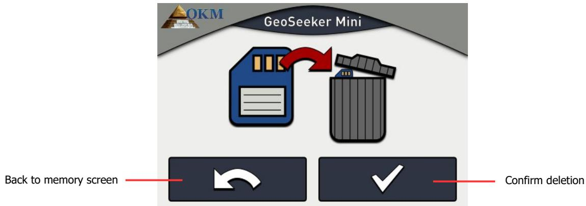
Figure 5.13: Delete stored measurement
