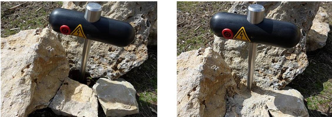
Figure 8.5: Drilling a hole and refilling it for the electrode
