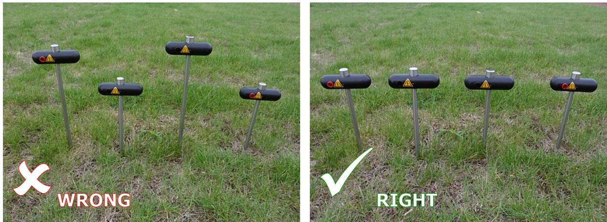
*Figure 8.2: Electrodes have to be equally set into the ground*
