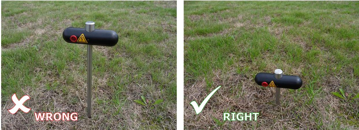
*Figure 8.1: Electrodes need good electrical ground contact*
