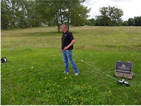
2. Unroll the cable of the first Voltage Cable Drum completely by laying it out in a straight line.
