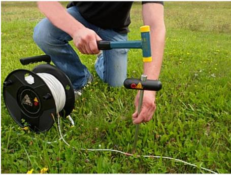
4. Put the Power Electrode next to the cable marker into the ground as deep as possible. Use a hammer if necessary.
