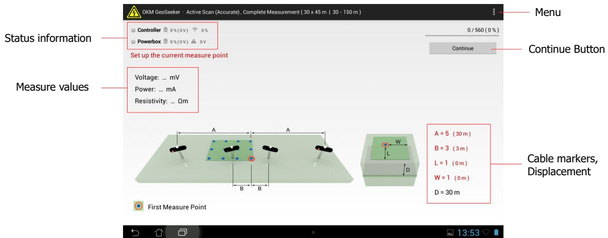
Figure 5.9: New Measurement - Arrangement of electrodes
