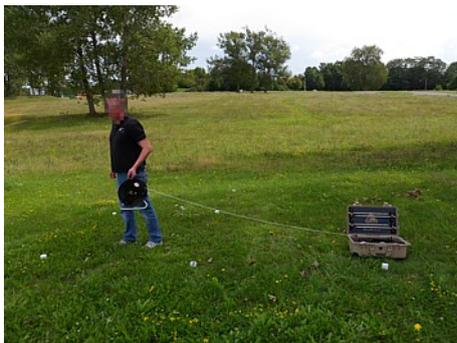
3. Unroll the cable of the Power Cable Drum by moving away from the Power Box until you reach the cable marker indicated by the Android application of your Tablet PC.
