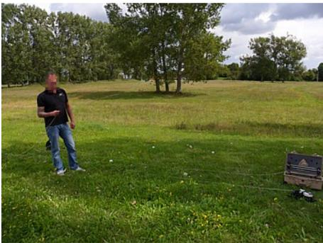
3. After reaching the end make a U-turn and bring back the cable to the cable marker indicated by the application of your Tablet PC. Unrolling the cable completely is necessary to get the right order of the cable markers and makes it easier to rearrange the electrodes afterwards.
