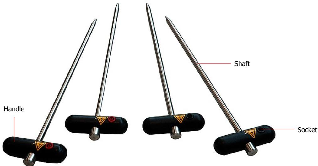
Figure 4.1: Elements of the electrodes
