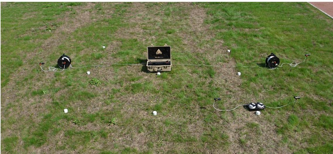
*Figure 7.7: Arrangement of electrodes during Active Scan (Quick)*
