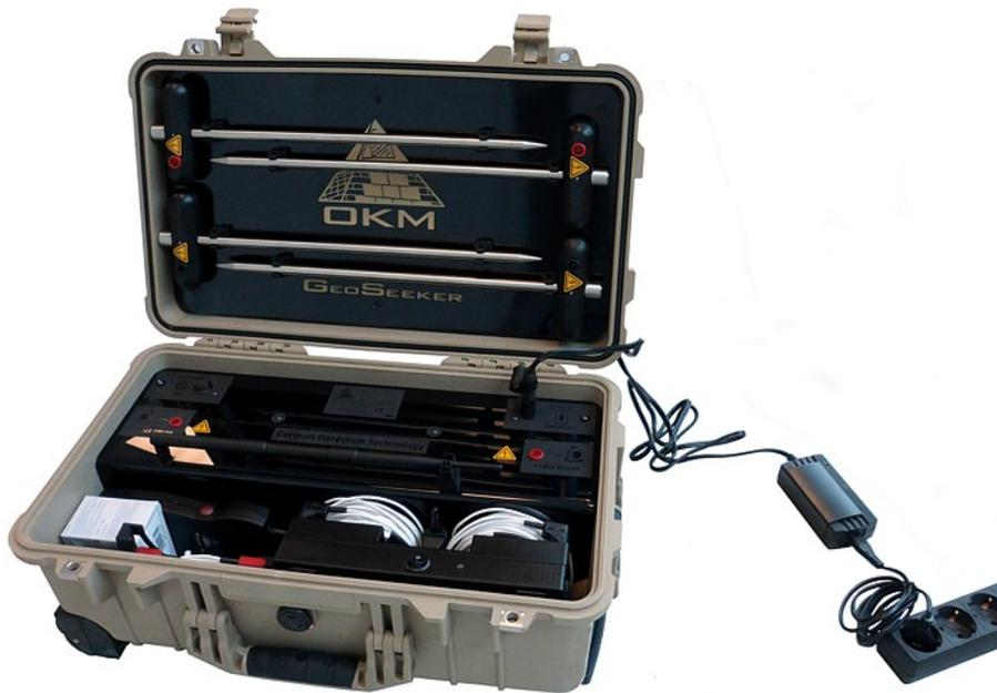
*Figure 6.5: Connecting the Power Box Charger*
