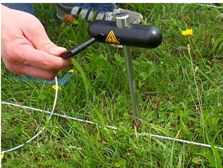
5. Connect the cable of the Voltage Cable Drum with the Voltage Electrode.
