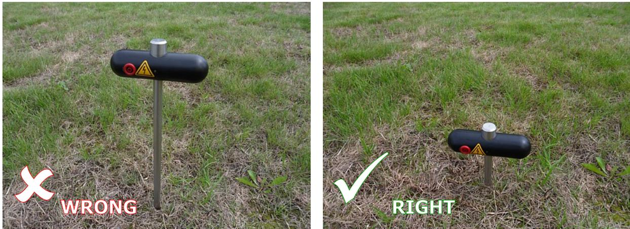
Figure 9.1: Electrodes need good electrical ground contact
