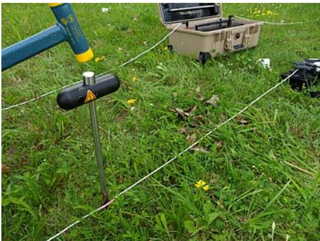
4. Put the Voltage Electrode next to the cable marker into the ground as deep as possible. Use a hammer if necessary.
