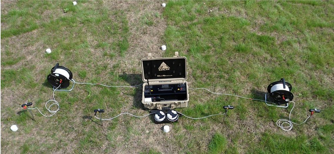
*Figure 7.6: Arrangement of electrodes during Active Scan (Accurate)*
