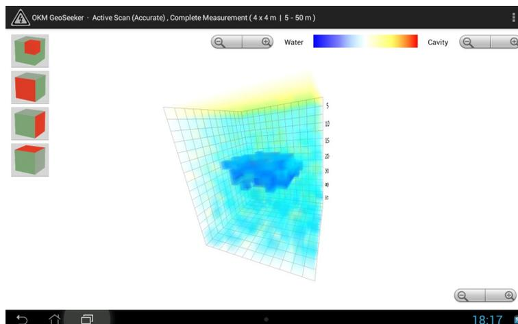
Figure 8.2: Graphical 3d representation of an active scan
