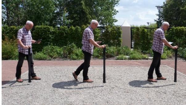
Figure 6.2: Probe should always point downwards and should not be turned
