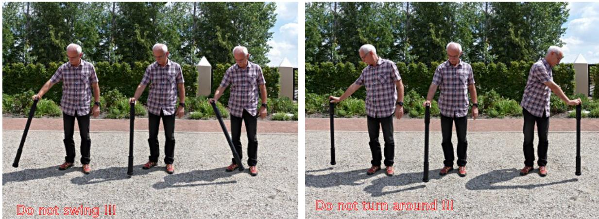
Figure 6.3: Pivoting or turning of the probe falsifies the measurement
