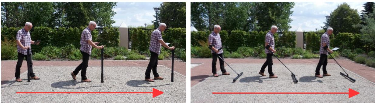
Figure 6.5: Ground Scan in vertical and horizontal mode
