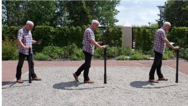
Figure 7.5: Probe should always point downwards and should not be turned
