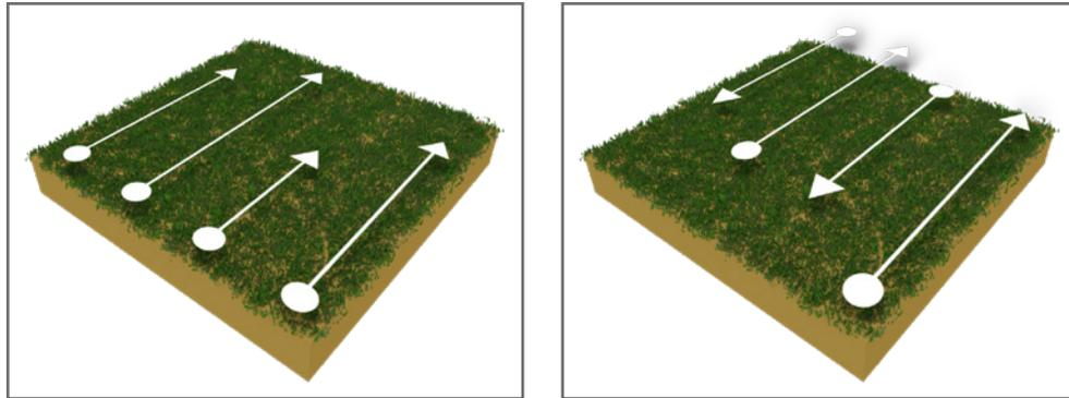
Using different walking speeds throughout the scan lines will cause displacements within the scan field. As a matter of fact, a potential target can get cut into several small pieces or completely lost because it was missed out. Later on, when the data is downloaded for further analysis, speed errors can make a target completely unidentifiable.
