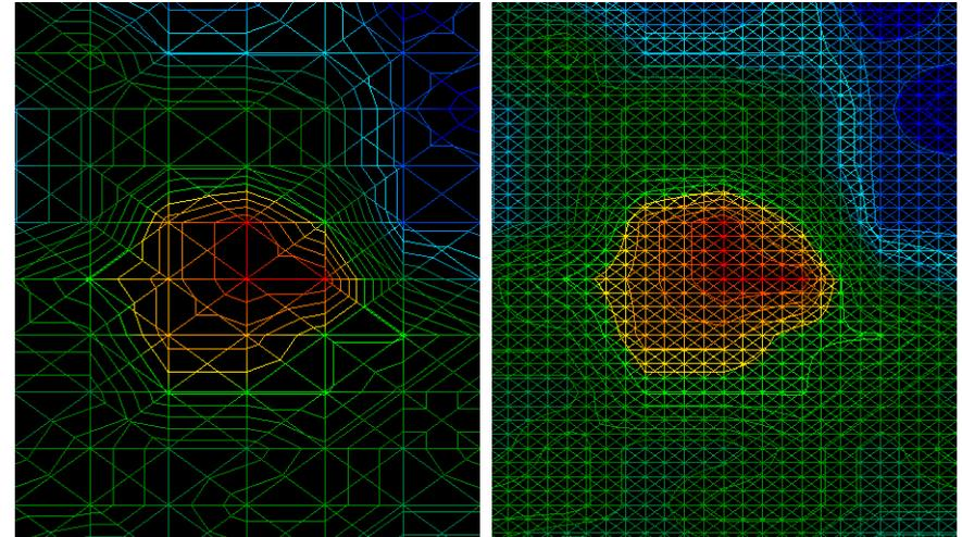
*Comparison: few impulses (left) and many impulses (right) at the same length of scan line. The second scan (right) shows more details and allows to detect even smaller objects.*
