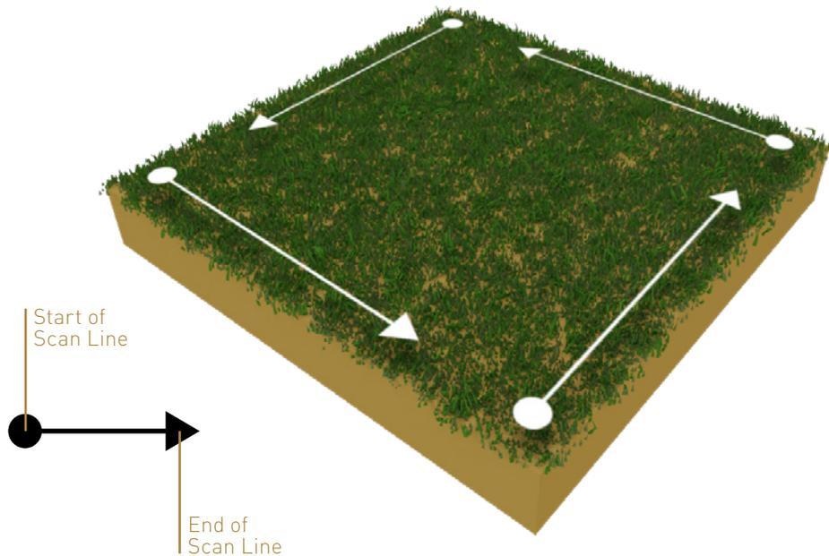
The scan lines may be performed in Parallel or Zigzag scan mode. The number of impulses (measure values) which are recorded during the first scan line can be adjusted individually depending on the length of your scan field.
